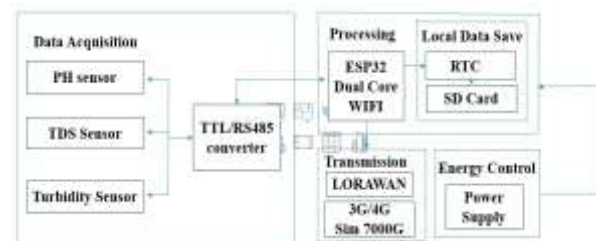
Fig.1. Block diagram water quality monitoring system
